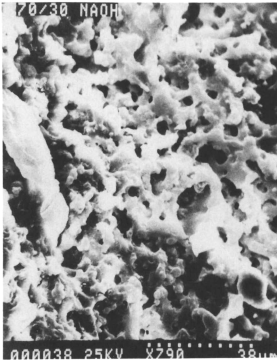
Figure 7. Scanning Electron Micrograph of a 70/30 (PLA/EVAc) Blend After Base Catalyzed Hydrolysis.
